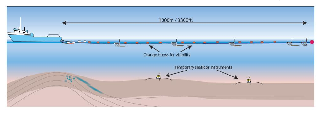
From June 24 to July 3, 2025, a geophysical imaging survey will take place off the coastline of West Hawai`i, mapping the electromagnetic conductivity of the sub-seafloor to locate possible deep, brackish or freshwater reservoirs beneath the ocean.
