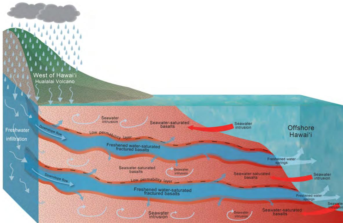
492 **Fig. 5. Fresh groundwater onshore to offshore transport mechanism.** Illustration showing
