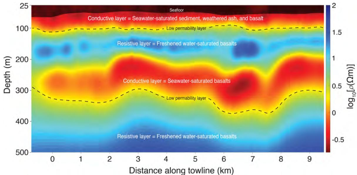
471 **Fig. 3. Line 3 North inversion model.** Model showing the electrical resistivity structure of line
