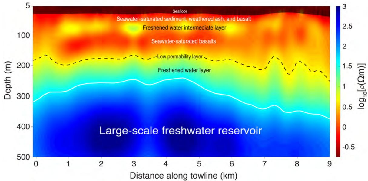
480 **Fig. 4. Line 2 South inversion model.** Model showing the electrical resistivity structure of
