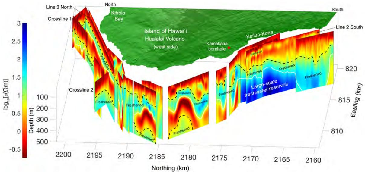
459 **Fig. 2. Multilayer electrical resistivity formation offshore the Island of Hawai'i.** Fence di-
