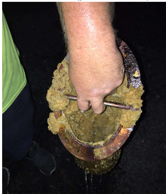
Sponge fouled pipeline at KPLG tenant's farm at HOST Park. (photo credit BOM)
