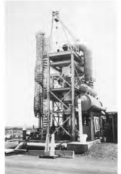
The Heat and Mass Transfer Scoping and Test Apparatus experiment is housed in a 30-foot tower within the NELH compound.
