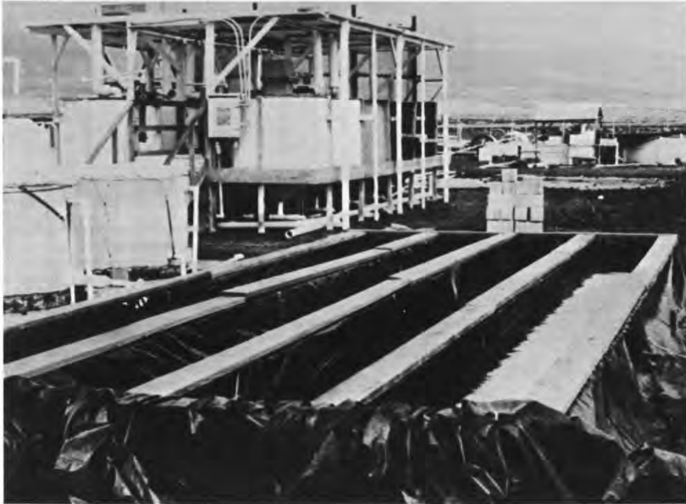
Troughs used to investigate algal removal of excess nutrients from returning seawater.
