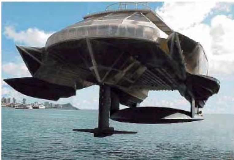
PACIFIC MARINE, INC. Unique hull design of midfoil ship, visible as vessel is suspended from a crane.
