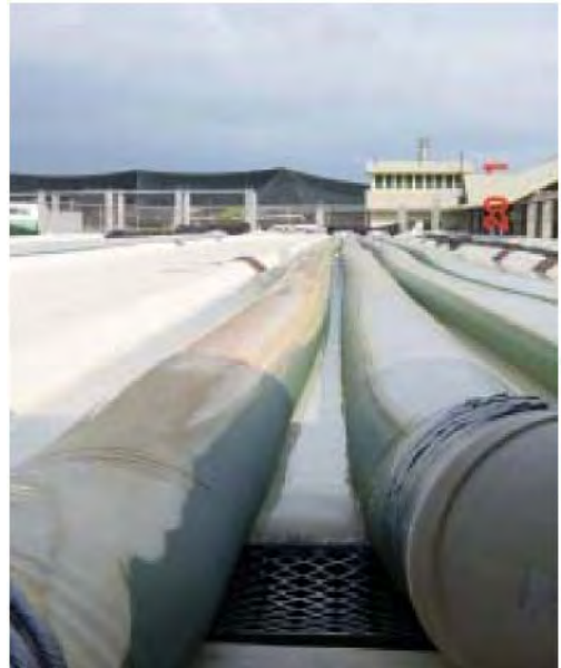
The Aquasearch Growth Module is a commercial-scale closed photobioreactor used to culture microalgae.
