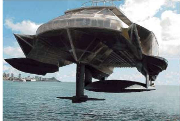
PACIFIC MARINE, INC. Unique hull design of midfoil ship, visible as vessel is suspended from a crane over the ocean.
