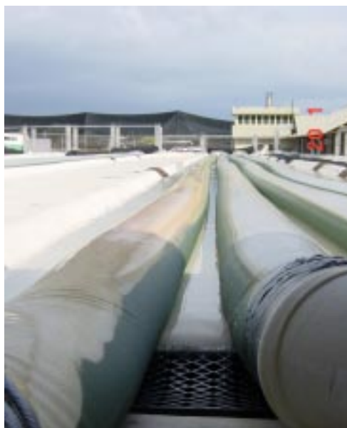
The Aquasearch Growth Module is a commercial-scale closed photobioreactor used to culture microalgae.
