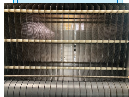
Above: Titanium foil plates stack as seen on prototype SWAC unit at Makai Ocean Engineering Lab in HOST Park. Photo courtesy of MOE.
