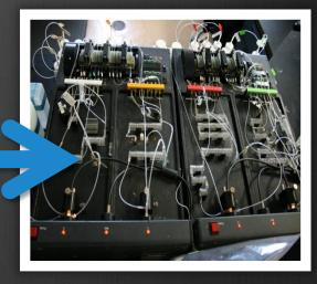
Nutrient concentrations analyzed via segmented flow auto-analyzer
