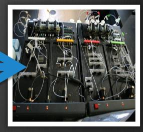
Nutrient concentrations analyzed via segmented flow auto-analyzer
