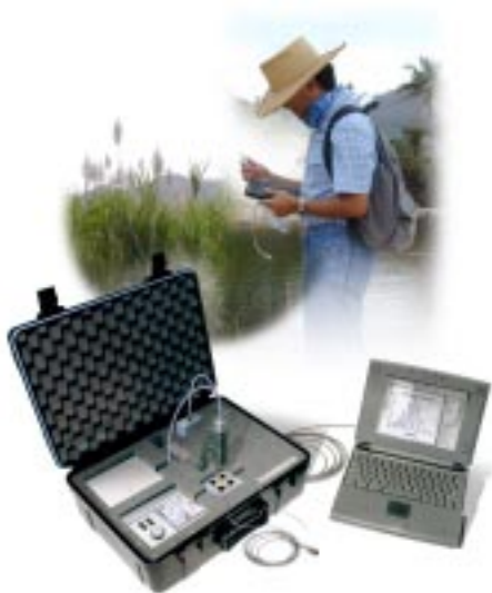
TREX ENTERPRISES, INC. Sensor for Pesticide Monitoring Based on a Porous Silicon Biosensor.
