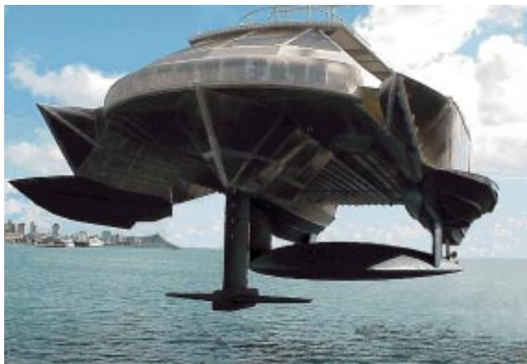
PACIFIC MARINE, INC. Unique hull design of midfoil ship, visible as vessel is suspended from a crane.
