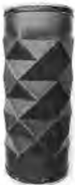
LEFT & BELOW: Structural Solutions-- Prebuckled Cylindrical Hull
