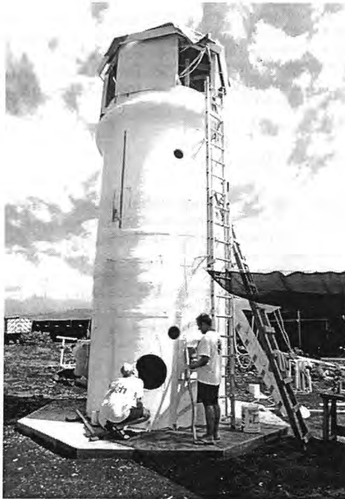
The "hurricane tower" experiment tested a new method of freshwater production from seawater.
