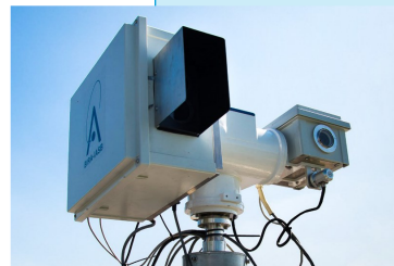
Above: Optical head of the MAX-DOAS instrument curtesy of BIRA
