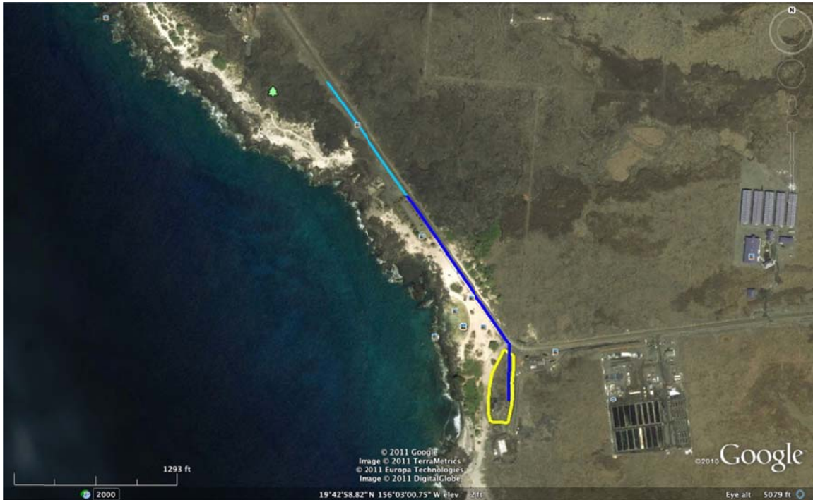
Figure 12. OTI Percolation Trench proposed route. Yellow polygon is the OTI OTEC site; Dark blue line is solid pipe to transfer DSW past Wawaloli Beach Park. Light blue line is the infiltration section.
