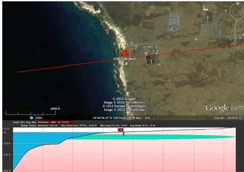
Figure 17. Plume Cross section, SSW injection at -100 to -150 feet. Red line marks surface intersection of profile.
