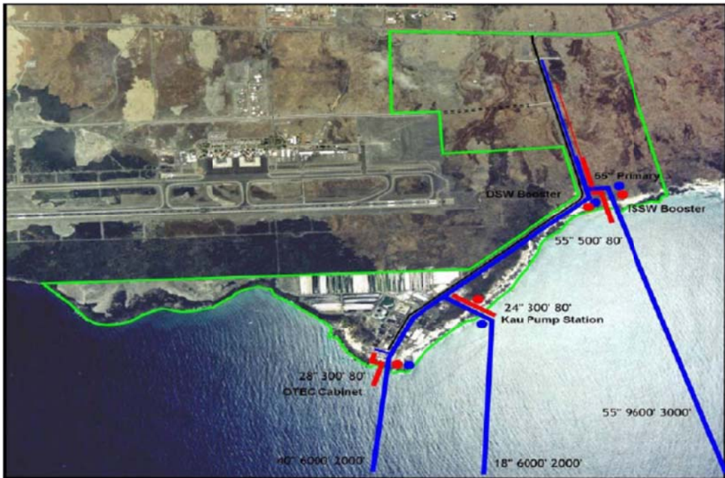
Figure 1 – NELHA Offshore Intakes and Distribution Pipelines
