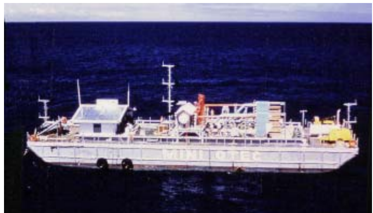
In 1979 the Mini-OTEC project at Keahole Point made world history as the first net power-producing plant to use the OTEC process, invented by French engineer Jacques D'Arsonval nearly 100 years before.
